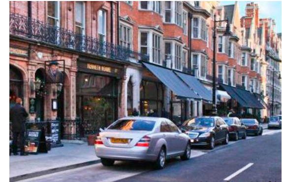
Mount Street, Mayfair; Paved car parking to exaggerate width of footpath
